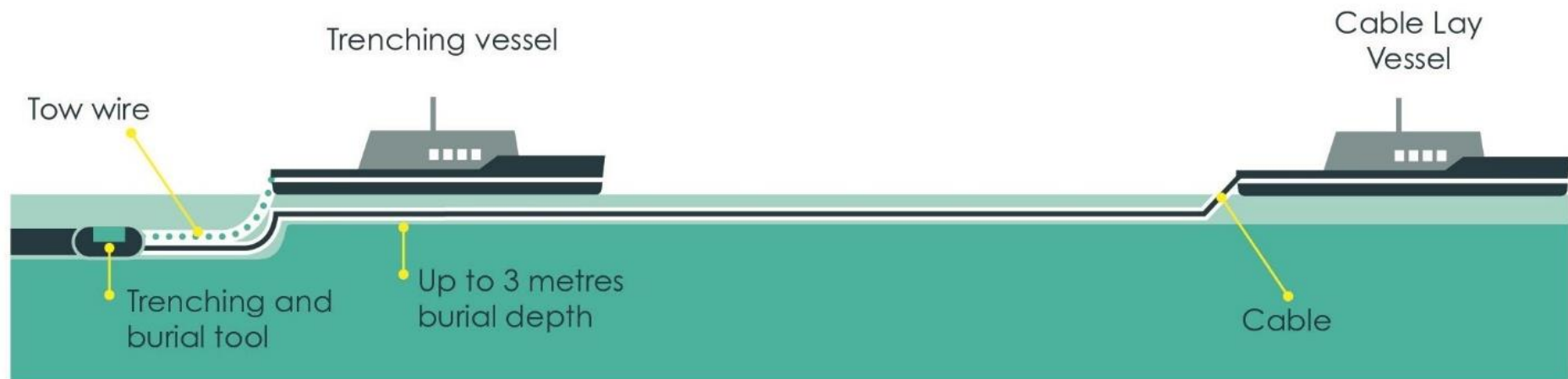
Plate 6.9 IAC, Interlink and export cable laying vessel and trenching vessel
